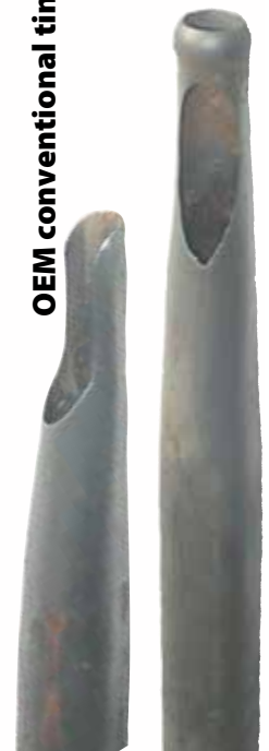
A JRM DILLENNIUM® tine with Severe Timing Problem
